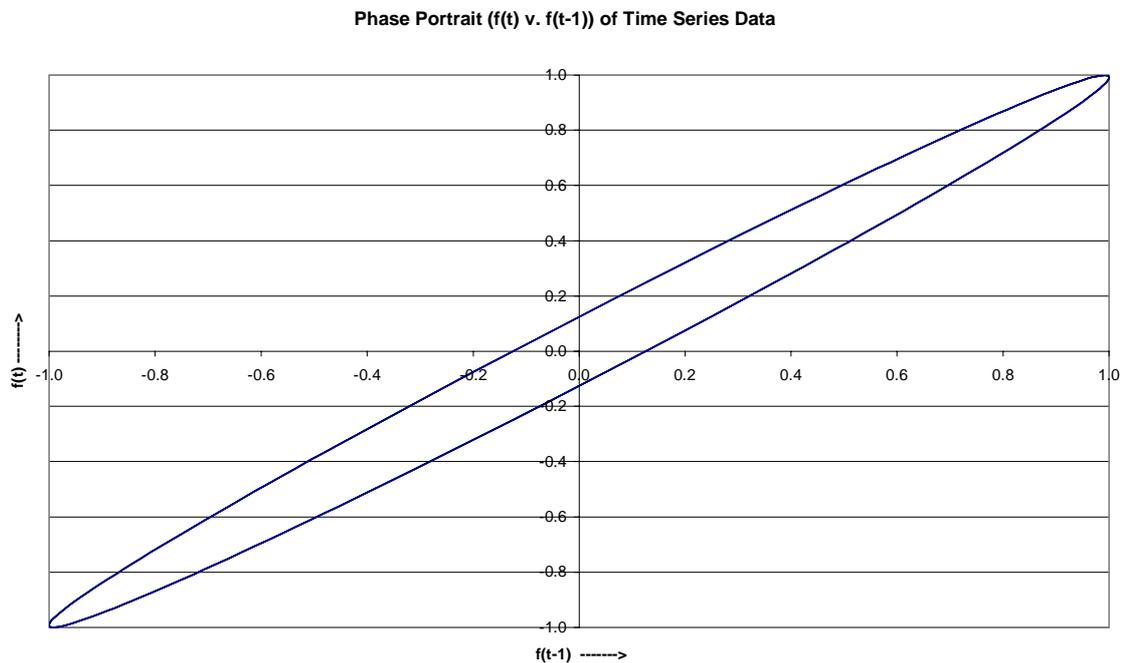
Fig 3b: A phase portrait is simply a plot of a current value,  $f(t)$ , against the preceding value,  $f(t-1)$ . For this time series, the result is a regular ellipse. Successive elements of the time series describe trajectories around this ellipse. Consequently a knowledge of this ellipse's properties is sufficient to predict  $f(t+1)$  from  $f(t)$ .
