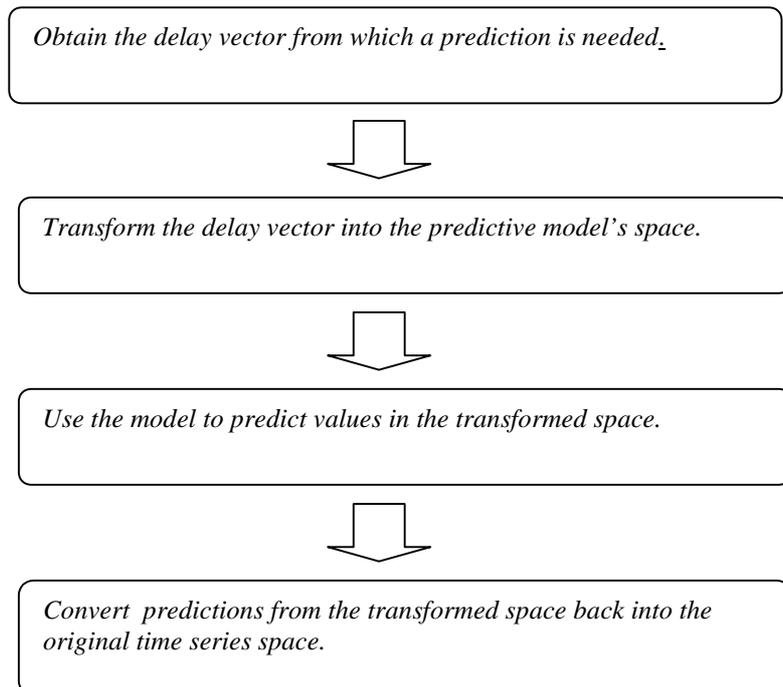
**Fig 5 -- Flow chart, showing the use of transformations for modelling and prediction.**
